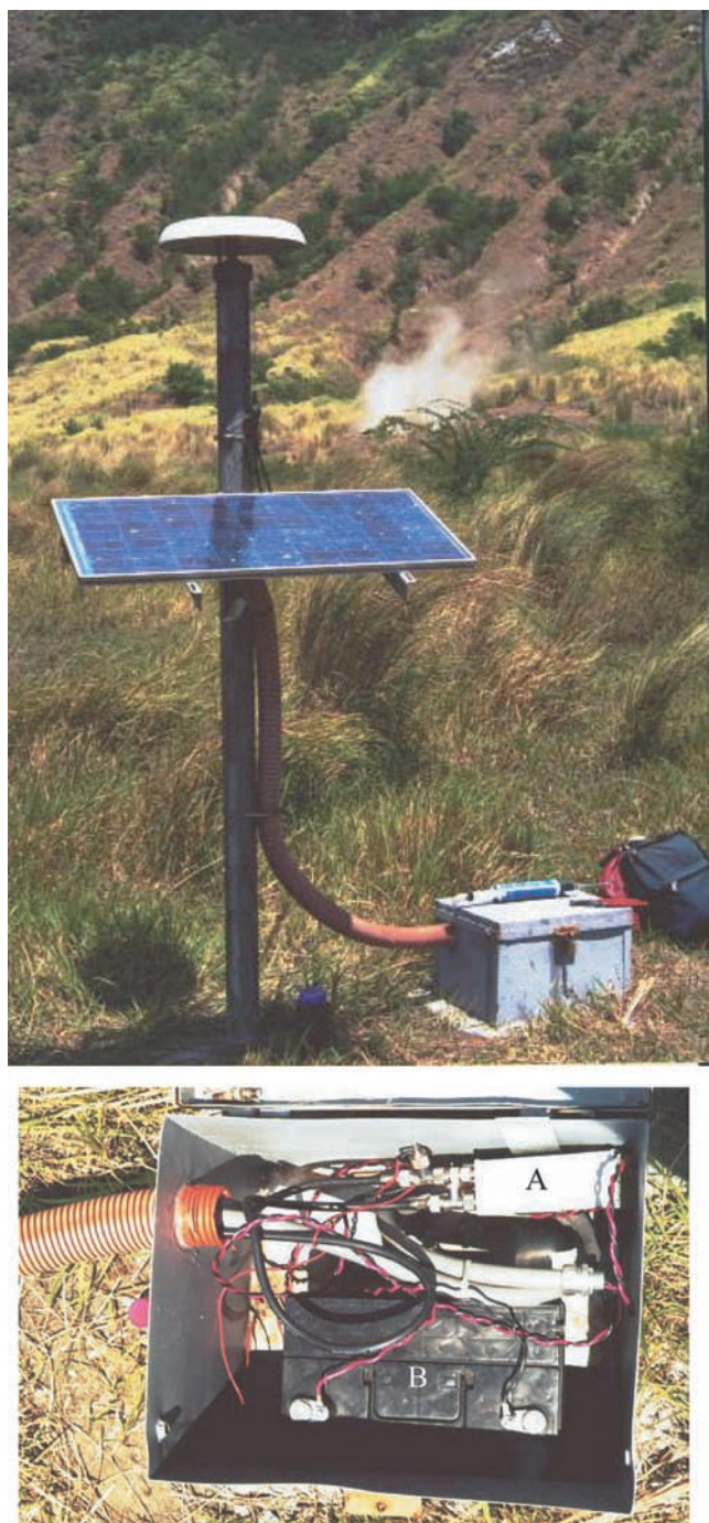
Figure 2. Single-frequency site set-up. Shown is site TV12, within the Main Crater. Contents of the stainless steel box include CMC GPS receiver housed together with FreeWave radio modem (A), and deep cycle battery (B). (Photographs by M. Hamburger.)
