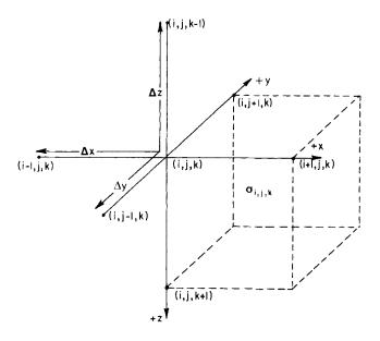
Fig. 1. Stencil depicting the indexing scheme used for the integrated finite-difference discretization (adapted from James, 1985).
