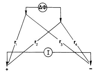
Fig. 5. An arbitrary dc resistivity electrode array.
