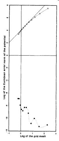
FIG. 4. Log of the Euclidean error norm of the potential versus log of the grid mesh for a uniform half-space. Results without singularity removal are represented as a dashed line; those with singular error removed are dotted. The unbroken line, having slope 2, shows the favorable comparison between actual and expected convergence with refinement of the grid.
